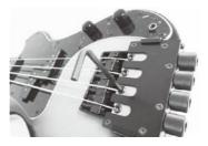
3) Next, pull the string on the head side, then loosen the M6 hex screw on the head side to remove the string.
